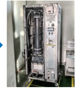
Paint booth recycling filtration equipment
