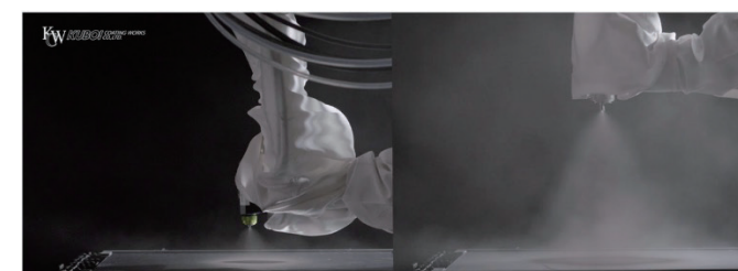
Spraying by the high transfer efficiency paint application & coating system (left) and by a typical coating system (right)
